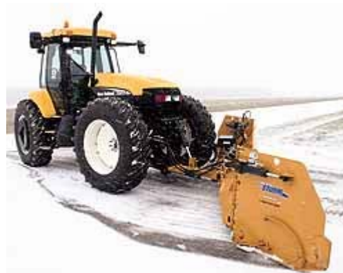
DeKalb County Airport employee Gene Powell operates the airport's new New Holland tractor, using a 14-foot blade with wings that open to clear a 21-foot swath of snow. The tractor was delivered to the airport this week, along with a snow blower and tracked Bobcat. Before acquiring its own equipment, the airport contracted for snow removal. (Bill Gisel)
